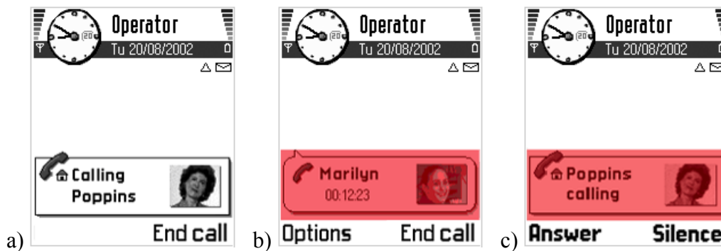
Figure 96: Phone application examples: a) Creating an outgoing call b) Active call going on c) Incoming call alerting
