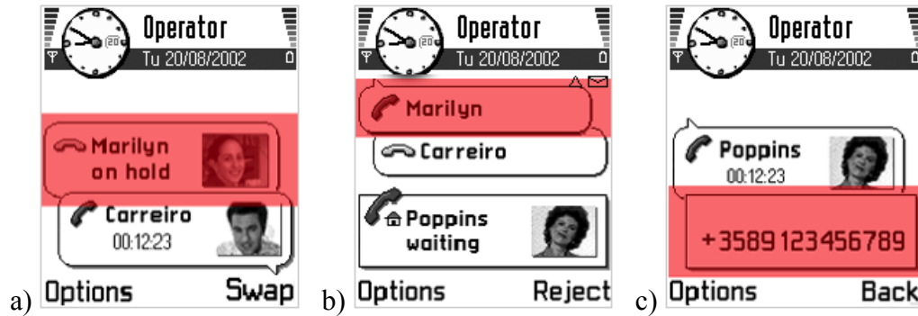
Figure 97: Phone application, multi-call cases: a) One call active, another on hold b) One active, one held, one waiting call c) User is entering a number while another call is active
