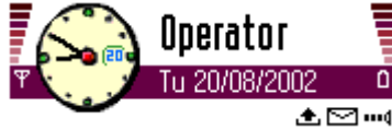
Figure 73: Signal and battery indicators on the sides of the status pane. Other status indicators are visible below the navi pane.
