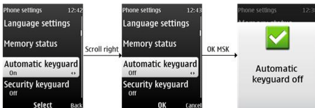
Figure 27: Example of UI flow using navigation key shortcuts with setting
