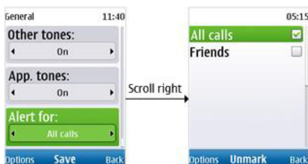
Figure 33: Example of UI flow where the navigation key opens another UI state
