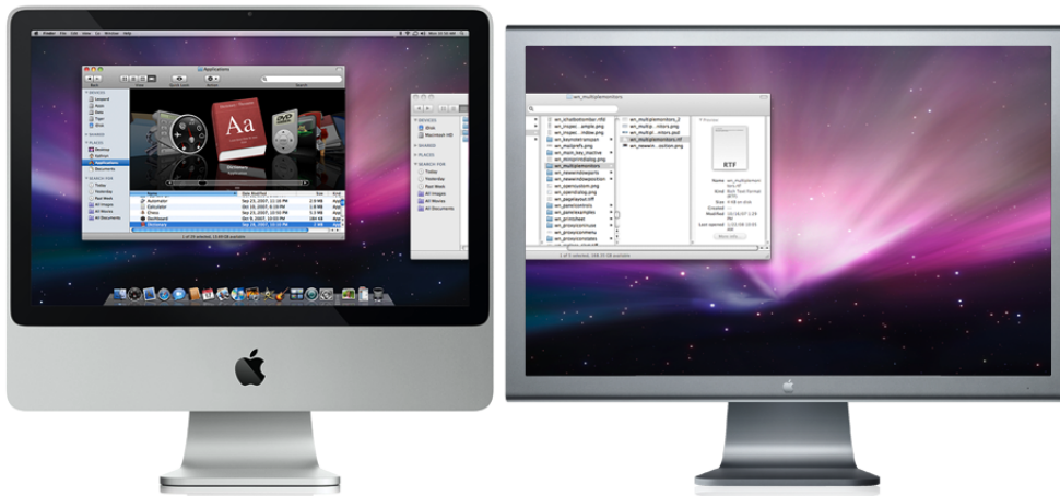
Figure 14-33 Appropriate placement of a new window on a system with multiple monitors (the user moved the first window to span the screens)
